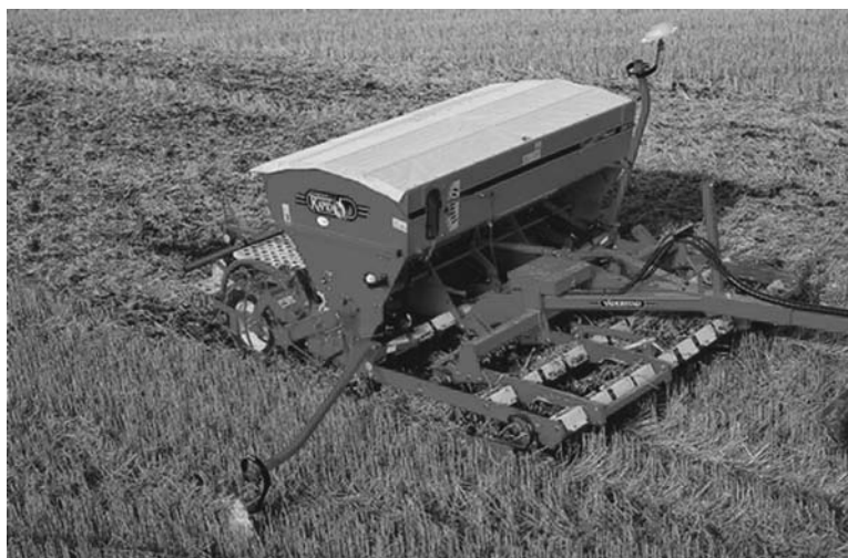
Fig. 9.1.2. Modern drills can go from stubble to drilled crop in a single pass (photo courtesy of Vaderstad Verken AB). For color details, please see color plate section.
